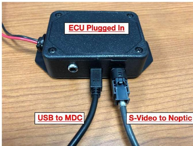
Step 3: Your ECU should look similar to the picture to the left. Once the Type-B Mini USB is plugged into the ECU, plug the Type-A USB End into the MDC. Your setup should now look similar to the below picture.
